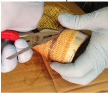
4. Every wrap you make down the pipe after that initial wrap needs to be  $\frac{1}{4}'' - \frac{1}{2}''$  of overlap. This also depends on if you are trying to wrap a pipe that curves. If the pipe has a drastic curve you may want to overlap more to make sure you do not create a bare spot that has not been covered with heat wrap. Our wrap is designed to disperse heat across the covered area and not create hot spots on the pipe if you have too much of an overlap.
