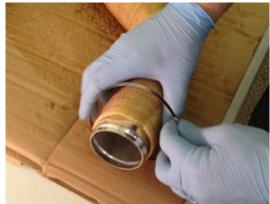
After reinstalling the pipe start the engine, while the engine is running the heat wrap will start the "Set up" process and may smoke or steam for short period of time but this is completely NORMAL.
