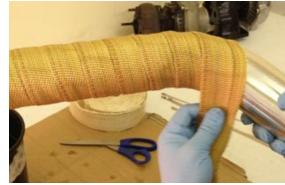
5. Finish the section of wrap by cutting of any excess wrap and securing your work in place with another Thermal Zero Stainless Steel Zip Tie.
