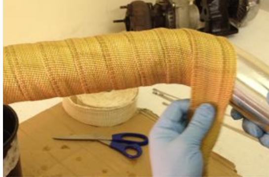
5. Finish the section of wrap by cutting of any excess wrap and securing your work in place with another Thermal Zero Stainless Steel Zip Tie.
