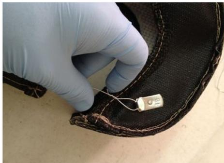
Now install the blanket around the exhaust side of the turbocharger and snug it down by hooking your twisted mechanics wire around the opposite hook on the turbo shield.
