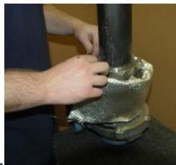
a. NOTE!!! If you are using an internal wastegate you will have to make a hole in both the aluminumized and white heat wrap to be able to hook up the lever.
