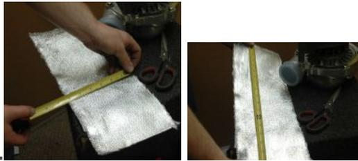
4. Take the aluminumized wrap. Along both of the long sides of the wrap make a series of 1/4" cuts approximately 1/2 inch from the edge of the material and about 1 inch apart.
