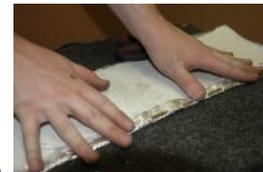
6. Then fold the aluminumized shielding lengthwise along the stainless tie.
