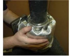
9. Cut the stainless ties to length and smooth the edges to prevent a sharp point.
